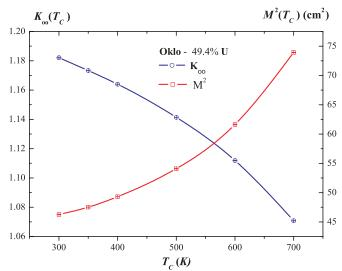
FIG. 4. (Color online)  $T_C$  dependence of  $K_{\infty}(T_C)$  and  $M^2(T_C)$  for a core containing 49.4 vol.% of uranium in the present-day dry ore and a water content of  $\omega_{\rm H_2O}^0 = 0.355$  at  $T_C = 300$  K and  $P_C = 0.1$  MPa. Calculations using code MCU-REA [44,45].
