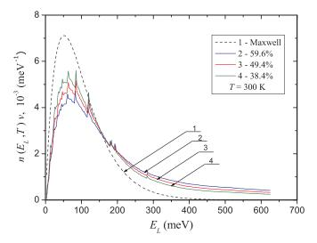
FIG. 5. (Color online) Neutron spectrum in the bare fresh core RZ2 at different initial uranium concentrations (water content  $\omega_{\rm H_2O}^0 = 0.355$ ). Calculations using code MCNP4C [44,45].
