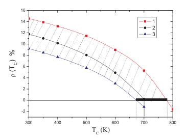
FIG. 3. (Color online) Power effect [44,45]. Dependence of reactivity  $\rho$  (in %) of the fresh core of the Oklo reactor on temperature  $T_C$  at a pressure of  $P_C=100$  MPa for three different initial compositions of the active core and different proportions of water: 1: 49.4 vol.% U in ore,  $\omega_{\rm H_2O}^0=0.455$ ; 2: 49.4 vol.% U in ore,  $\omega_{\rm H_2O}^0=0.405$ ; 3: 38.4 vol.% U in ore,  $\omega_{\rm H_2O}^0=0.355$ . Calculations were done using code MCU-REA.
