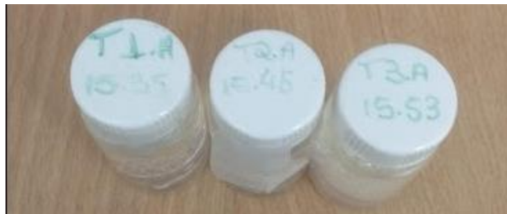
Figure 7 Vials with sampled water and OptiFluor-O cocktail
