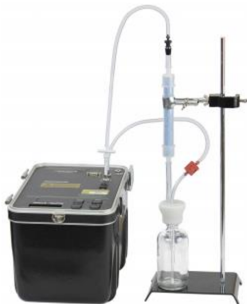
Figure 2 Rad7 - water measurement setup
