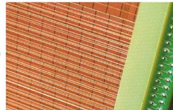
Pad side of an inner readout chamber, showing the segmentation into small pads and the wire grids on top
