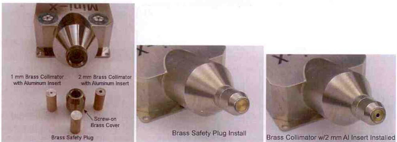
Figure 4. Left photo shows the Mini-X collimators, safety plug, and cover. The middle photo shows the safety plug installed in the cover and attached to the Mini-X. This configuration meets the radiation requirements discussed in Section 1.2. The Mini-X ships from the factory in this configuration. The right photo shows the collimator installed in the cover.
