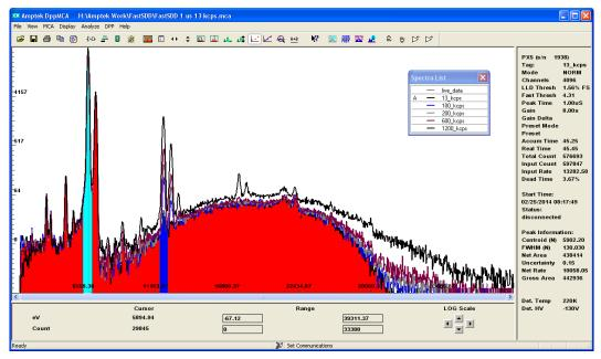
The plot below shows spectra taken at 200 kcps with the FastSDD, with peaking times from 0.1 to 4.0  $\mu$ s with a fixed  $T_{Fast}$  of 50 ns . Note that there is negligible change to the overall spectrum, and in particular, that the sum peak intensity is constant. The only changes are in the resolution of the photopeak and also in the acquisition time (not shown in the plot but the data were taken to fixed photopeak counts and thus for accumulation times from 4.5 to 25 sec).
