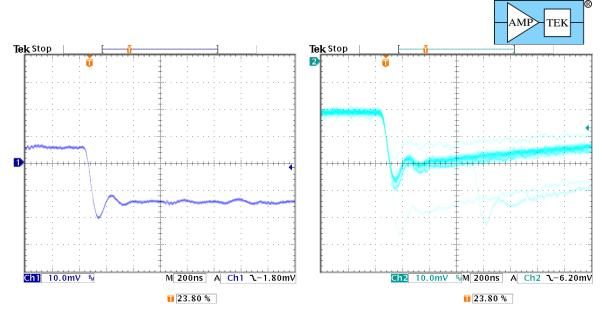
**Preamplifier risetime**. The plot on the left shows the trace from the preamplifier for a single pulse at a short time scale, while the trace on the right shows the AC coupled signal from several pulses.
