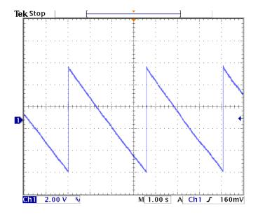
**Preamplifier output.** This trace also shows the preamp output but on a different voltage and time scale to illustrate the reset. The small steps from each signal integrate towards the negative rail, where a reset signal is generated. This results in a sawtooth of several volt amplitude. The period depends on the total current through the detector (signal current plus leakage current).
