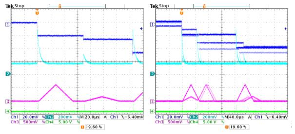
**Signals.** These traces show the preamplifier output (dark blue), the input to theADC (light blue) and the shaped output (magenta) for typical pulses. The trace on the left shows three pulses which are well separated in time. The plot on the right shows several different traces.
