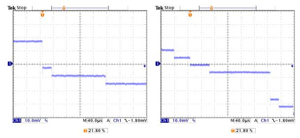
**Preamplifier outputs.** These traces illustrate typical output pulses with a SiPIN detector, measured using 5.89 and 22.1 keV X-rays. Each X-ray interaction results in a negative going step of ~1 mV/keV
