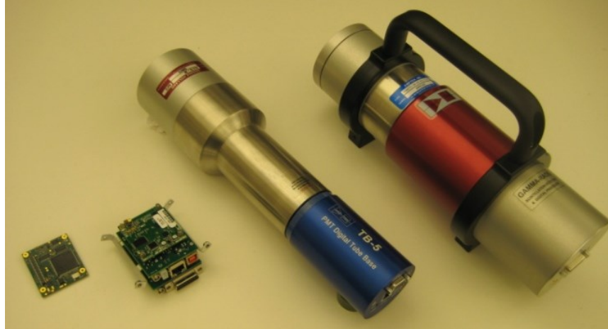
Photo showing, from right, (1) the Gamma-Rad5, a complete scintillation spectroscopy system; (2) the TB-5 digital tube base plugged into a scintillator/PMT; (3) the DP5G/PCG electronics assembly; and (4) the DP5G digital pulse processor for scintillation spectroscopy.
