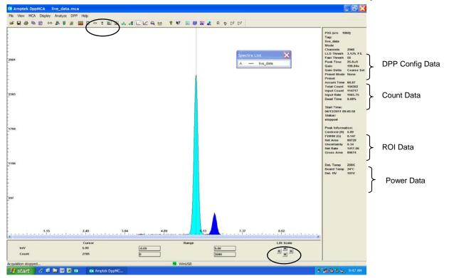
d. The primary data from the DP5 are the spectrum and the count rates. There are auxiliary outputs on the DP5. These are useful for interfacing the DP5 with other hardware. They are described in the DP5 user manual.
