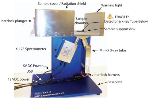
\*Beryllium windows damaged by improper handling will not be covered by the warranty.
