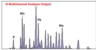
Trace 1 above shows the input to the DP5, which is the output from a reset-type charge sensitive preamplifier. This is processed by the analog prefilter producing the prefilter output shown in Trace 2. This is digitized and then processed digitally, producing the DP5's shaped output shown in Trace 3. Finally, the DP5 creates a multichannel anlayzer (MCA) type output spectrum shown in Graph 4.
