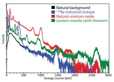
Measured γ-ray spectra of naturally occurring radioactive materials (NORM), an industrial 133Ba isotope, compared to natural background with no sources present.
