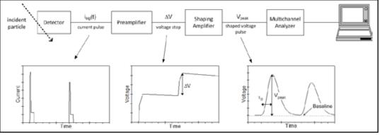
Figure 3. Complete Pulse Height Analysis System
