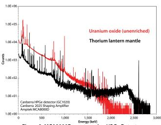
Figure 8. MCA8000D spectra using HPGe Detector
