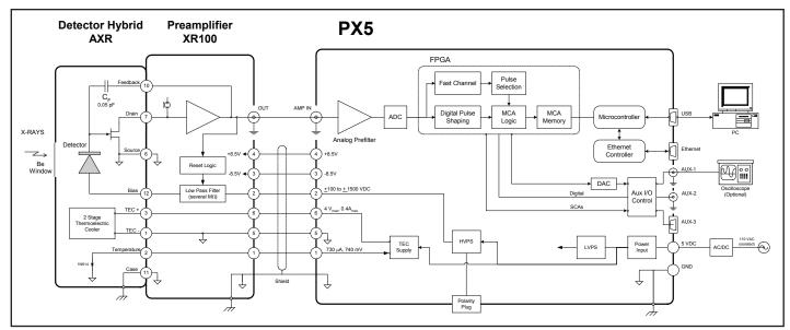
Block diagram of a typical system using the PX5 and an Amptek XR100SDD detector. Several different detector and preamp configurations are available from Amptek, Inc., with different pinouts and voltages.
