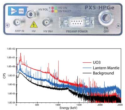
Spectra of low intensity material obtained with HPGe detector and a PX5-HPGe signal processor.
