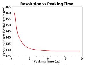
Figure 4. Resolution vs. Peaking Time for the SDD.
