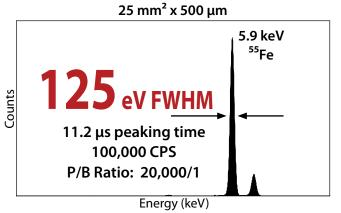
Figure 1. 55 Fe Spectrum with Silicon Drift Detector (SDD).
