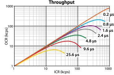
Figure 3. Throughput with the SDD. Due to the detector's smaller capacitance, a much shorter peaking time is used in the shaping amplifier without sacrificing resolution. Typically 9.6  $\mu$ s or less is used. This dramatically increases the throughput of the system.
