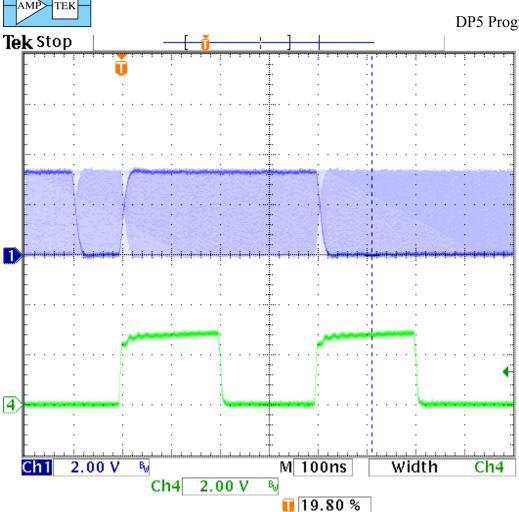
The timing shown is with the clock set to 20MHz. The strobe high and low times are 200nS, as is the minimum idle time between events (i.e. the strobe low time after the 2<sup>nd</sup> strobe, and before the 1<sup>st</sup> strobe of the next event.) In reality, this idle time is governed by the peaking time – the minimum peaking time @ 20MHz is 800nS, and therefore the minimum idle time at 20MHz is approximately 800nS. The actual idle time is governed by the configured peaking time.
