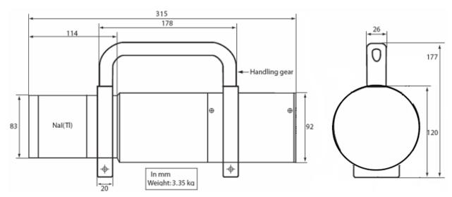
This is for the 76mmx76mm NaI(TI) scintillator, which is the most common. Contact Amptek for drawings of other configurations.
