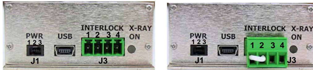
Figure 5. Showing the interlock disabled (left) and enabled (right).
