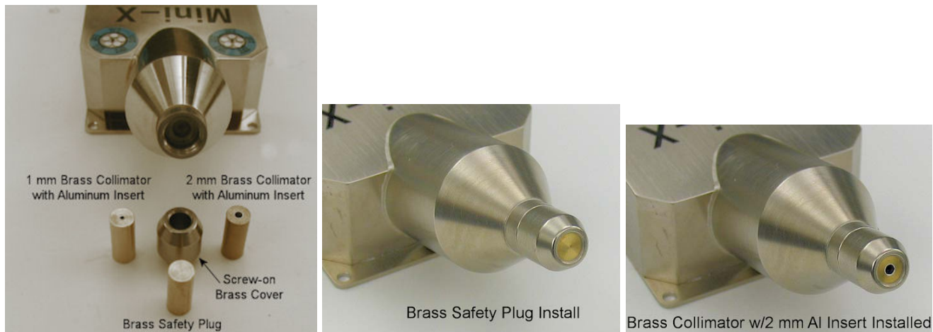
Figure 4. Left photo shows the Mini-X collimators, safety plug, and cover. The middle photo shows the safety plug installed in the cover and attached to the Mini-X. This configuration meets the radiation requirements discussed in Section 1.2. The Mini-X ships from the factory in this configuration. The right photo shows the collimator installed in the cover.
