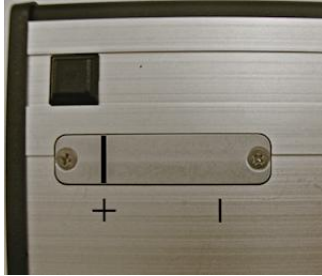
PX5 high voltage jumper set to positive for Si-PIN or CdTe detector.
