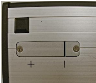
PX5 high voltage jumper set to negative for silicon drift detector (SDD)
