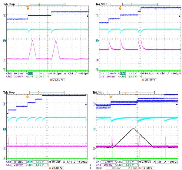
**DAC (analog) outputs**: The analog, DAC output is used to show diagnostic signals representing the waveform during the signal processing. In all these plots, the dark blue trace shows the preamp output and the light blue trace shows the ADC input.
