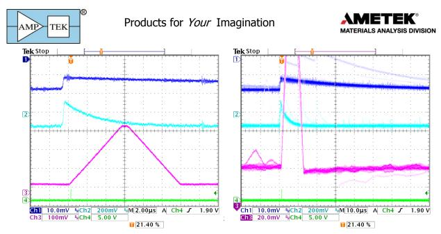
**Pole zero correction**: The traces above show signals from a detector with resistive feedback, in this case an HPGe detector with a 50 µs tail. The dark blue trace, the preamp output, drops exponentially to baseline rather than exhibiting the steps of the reset preamplifier. Circuitry in the DP5 cancels this tail (known technically as pole-zero cancellation) so that the light blue trace exhibits a strictly exponential recover, yielding the magenta trapezoid.
