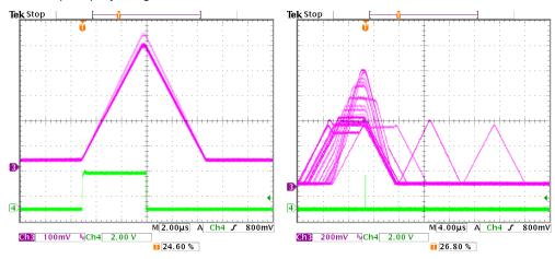
**Peak Hold**: The green trace on the left shows the peak hold signal, indicating when the logic was searching for the peak. **Pileup**: The green trace on the right is produced when two pulses pile-up, at the time of the peak of the second pulse.
