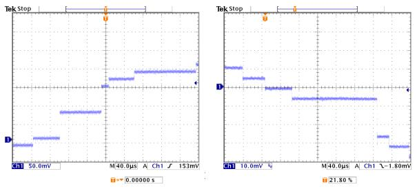
**Preamplifier outputs.** These traces illustrate typical output pulses with Amptek's X-ray detectors, which use reset preamps. The plot on the left is for a FastSDD<sup>®</sup> detector; each X-ray interaction results in a positive going step of ~3.7 mV/keV. One can distinguish the 5.9 and the 22.1 keV steps. The plot on the right is for a Si-PIN, which produces negative going pulses with a gain of 1 mV/keV.
