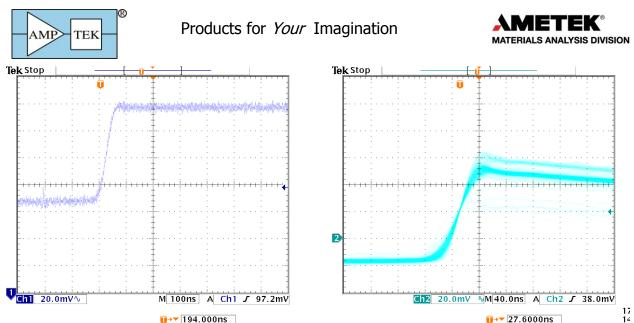
**Preamplifier risetime**. The plot on the left shows the trace from the preamplifier for a single pulse at a short time scale, while the trace on the right shows the input to the ADC from several pulses. These are for a FastSDD<sup>®</sup> with <sup>55</sup>Fe. The distinct traces for the  $K_{\alpha}$  and  $K_{\beta}$  energies are visible.
