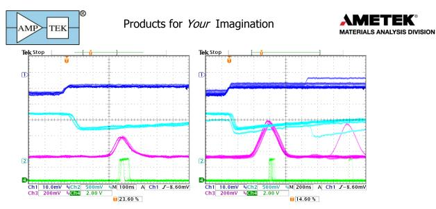
**ICR:** These traces illustrate the ICR (Incoming Count Rate) pulse. This is produced by a comparator operating on the fast channel. Any pulses which exceeds the fast threshold will generate an ICR pulse. This is used to produce the fast or input count rate and in the pile-up reject logic.
