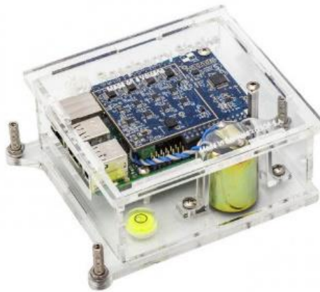
Fig 5. Raspberry Shake 4D contains a geophone, the blue RS4D board with three accelerometers, connected to a green RaspberryPi board computer [17].
